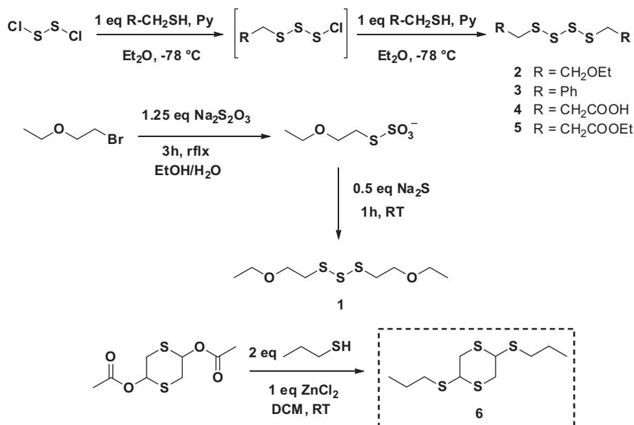
**Fig. 1.** General method employed for the synthesis of tri- and tetrasulfane derivatives based on previous literature reports. Chemical structures of compounds are shown.
